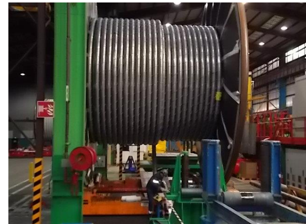
Flexible riser carcass in manufacture
